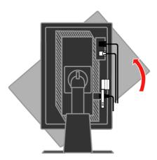
6. Place the cables through the Main Clip. Then fasten the clip.
